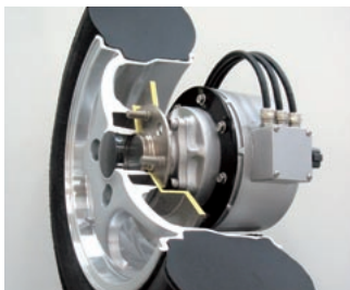
Axle Bearings with integrated In-wheel Motors
