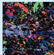
Treated by Fine Austenite Strengthening (FA) processing
