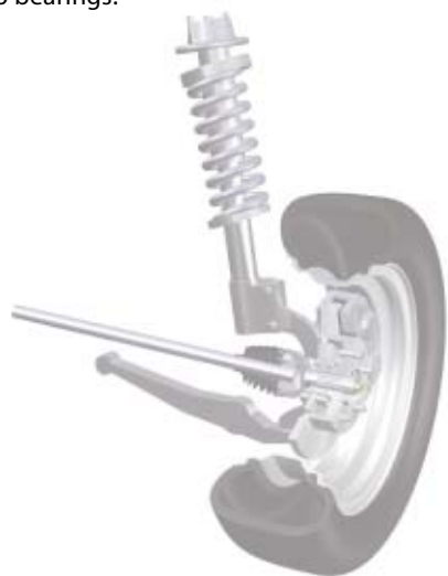
Fourth-generation hubjoint with wireless ABS sensor
